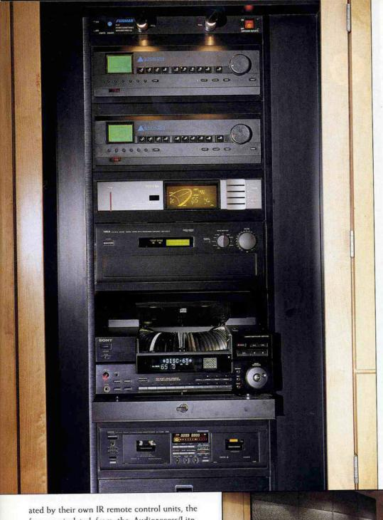
In addition to offering impressive audio and video to the media room, this equipment stack provides music and video to 11 other zones throughout the wholehouse system, which is controlled by Audioaccess and LiteTouch wall panels. Fabric panels on the back wall (below) deflect sound to the side walls of the theater.
